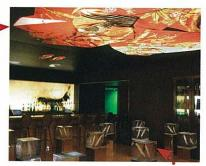
For the backlit fabric ceiling, dimmable TB 4.100K striplights were carefully located above kimono graphics to avoid backlighting the black portion of the fabric.
