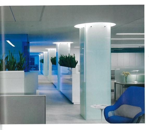
In the open office, linear fluorescent slot fixtures are the primary source. Linear LEDs in the ceiling plenum highlight the glass-cladded columns, accentuate the round ceiling cutout and provide egress pathway lighting.
